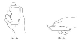
Fig. 1. Normal device orientation  $(o_n)$  with the display pointing upwards and alternative orientation  $(o_a)$  with the display pointing to the side (both seen from above).
